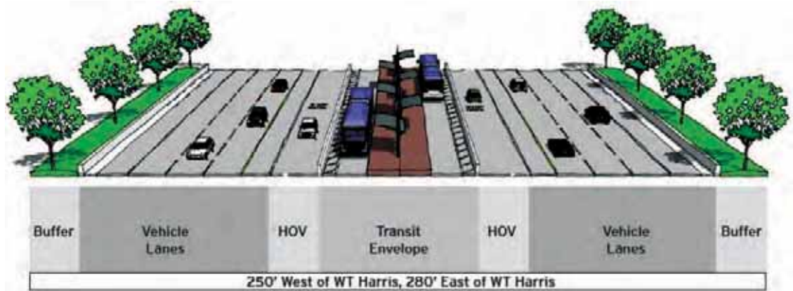
The previously proposed cross section for Independence Boulevard, including an envelope for general purposes, HOV lanes, and transit lanes.
